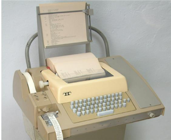
**Figura 6:** Máquina Teletype ASR-33 [26].
